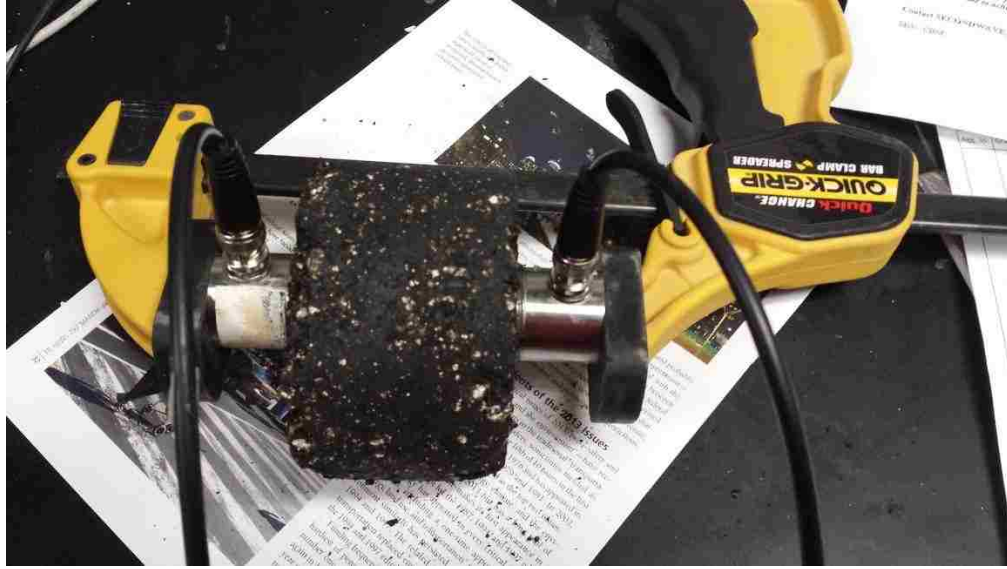
Figure 48. Sample fixed between two transducers
